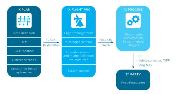
The PAS 880 system uses Phase One's intuitive software package designed to handle all aspects of photogrammetric project workflows, from flight planning to creating commercial format images.
