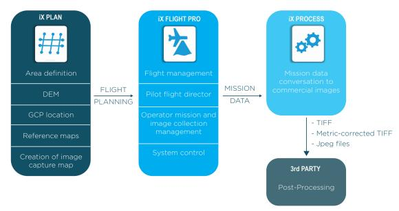
The PAS 880 system uses Phase One's intuitive software package designed to handle all aspects of photogrammetric project workflows, from flight planning to creating commercial format images.
