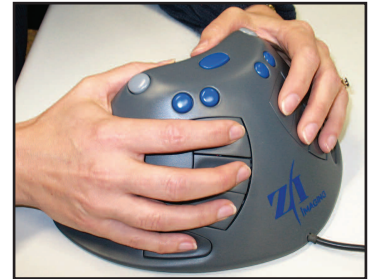
Intergraph’s Z/I Mouse provides photogrammetrists with an easy-to-use and precise manner to input data without the need for a digitizing surface.
