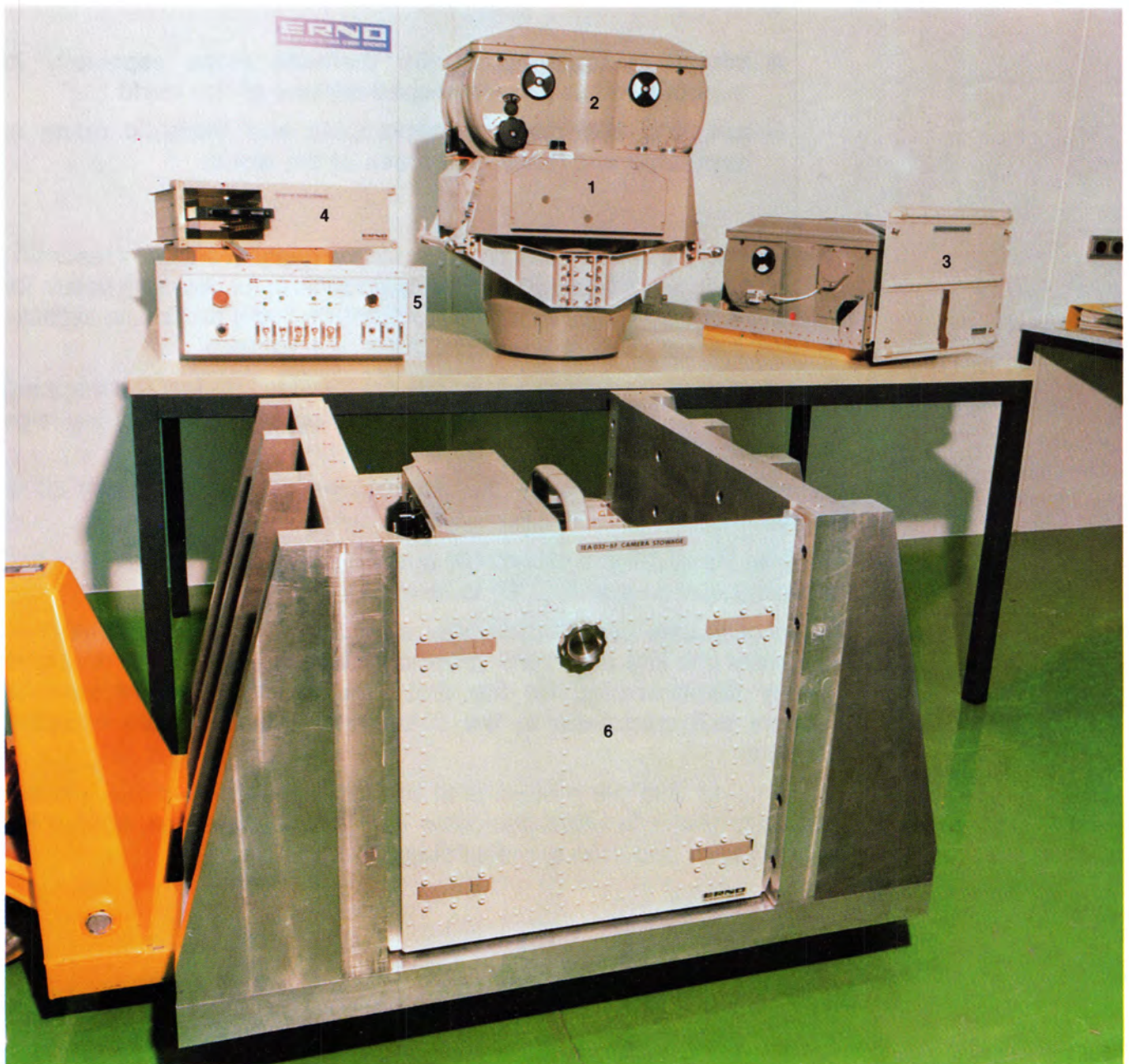
Metric Camera Flight Hardware: (1) Camera; (2) Film Magazine; (3) Film magazine in stowage container; (4) Filter in stowage container; (5) Remote Control Unit; (6) Camera Stowage Container. (Photo: ERNO)
