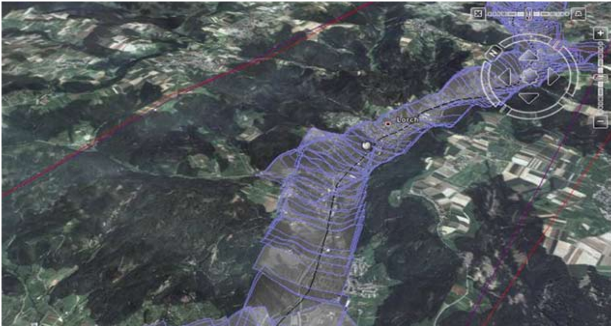
Z/I Mission includes 3D mission planning capabilities. This image shows the exposure centers at their precise position and the photo footprints projected onto the DTM surface exported into Google Earth.
