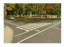
**Measurement between 2 Points** Distance, height, tilt, and azimuth can be measured by clicking two points on the PC screen.
