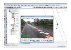
**Points, Polylines, Polygons** Points, polylines and polygons can be traced on the PC screen and registered as spatial information.
